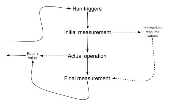
**Figure 3.2:** The default control flow of the DADT protocol. Solid lines represent the flow of control and dashed lines represent communication between stages.
