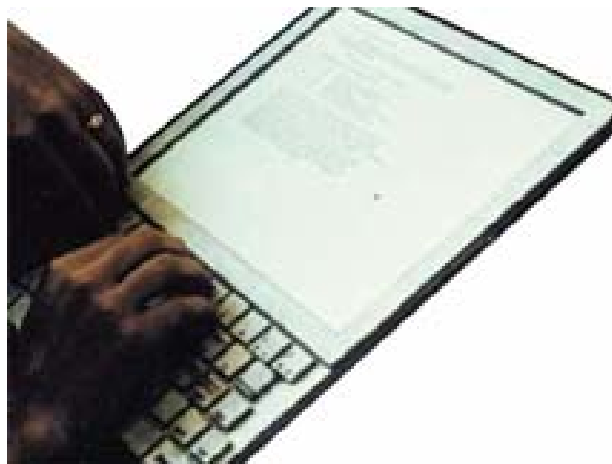
Figure 7-18 Dynabook Mockup provided by Larry Press [54]. While Kay's goal was a machine less than 2.5cm thick, the first version of the Dynabook, the "Interim" Dynabook was built using a desk-sized workstation.
