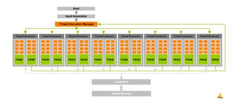
A GPU consists of several streaming multiprocessors (SMs) with a large shared memory. In addition, each SM has a local (and private) and small memory. Thus, GPUs cannot be classified as UMA or NUMA.
