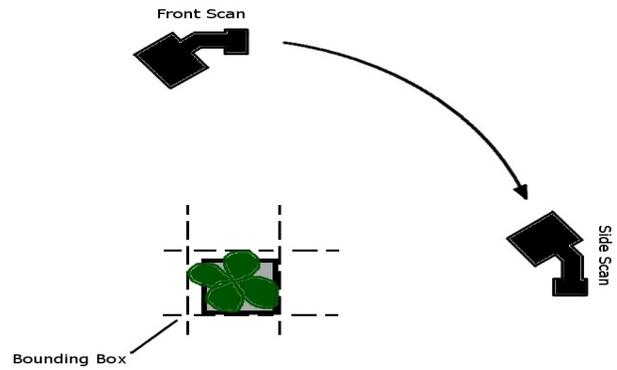
Figure 3. Pre-scan of plant from front and side
