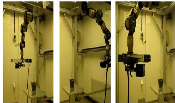
Figure 4. Scan head is rotated around plant to discrete positions
