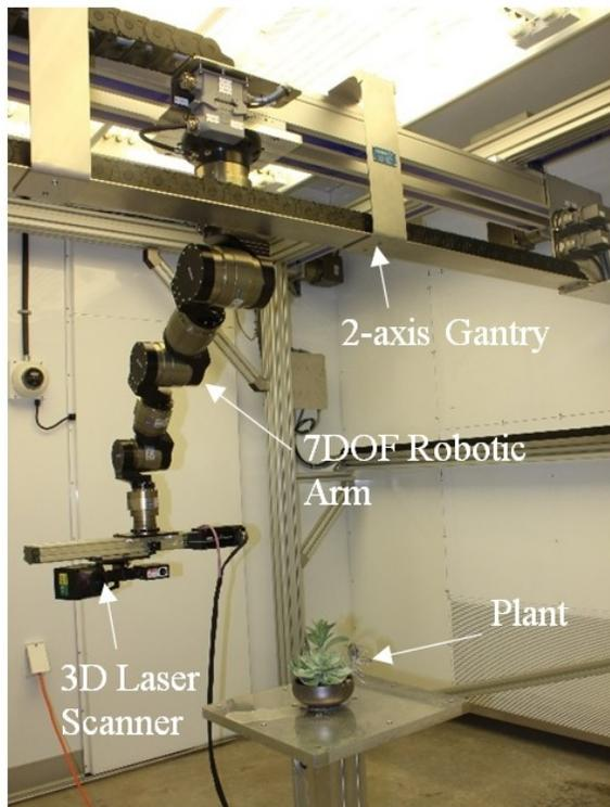
Figure 1. Robotic quantitative laser imaging platform (QLIP)
