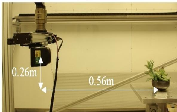
Figure 2. Scan head position relative to plant
