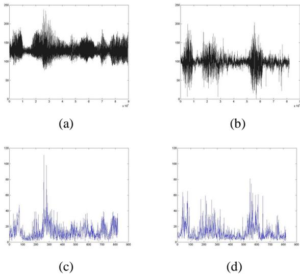
**Fig. 6.** (a) Original sound wave recorded from a 78RPM record player. (b) Recovered sound wave from groups of groove images. (c) Wave peak envelope of the original sound. (d) Wave peak envelope of the recovered sound.
