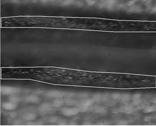
**Fig. 2.** The groove image captured directly using the 40X objective lens. Notice the shallow depth of field. Only two stripes (shown in highlighted areas) on opposite groove walls of same depth are in focus.
