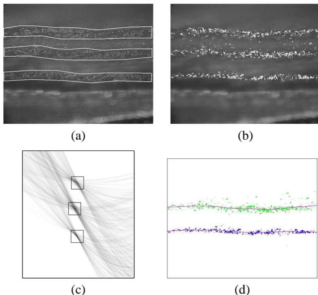
**Fig. 5.** (a) Groove image captured using 40X objective lens. Notice there are only three stripes (highlighted areas) on opposite groove walls of different depths that are in focus. (b) Locations of computed optical flow (white dots) for this area. (c) Results of Hough transform. The 3 square boxes indicates the 3 peaks that represent the 3 clustered lines. (d) Two segmented regions and their centroid lines.
