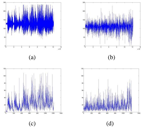
**Fig. 8.** (a) Original sound wave recorded from a 78RPM record player with audible pops. (b) Recovered sound wave from groups of groove images. (c) Wave peak envelope of the original sound. (d) Wave peak envelope of the recovered sound.
