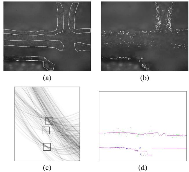
**Fig. 7.** (a) An image showing a damaged groove. (b) Positions of the computed optical flow. (c) Results of Hough transform. The 3 square boxes indicate the 3 clustered line regions. (d) Two segmented regions and their centroid lines. The missing parts has been filled in using the computed line parameters.
