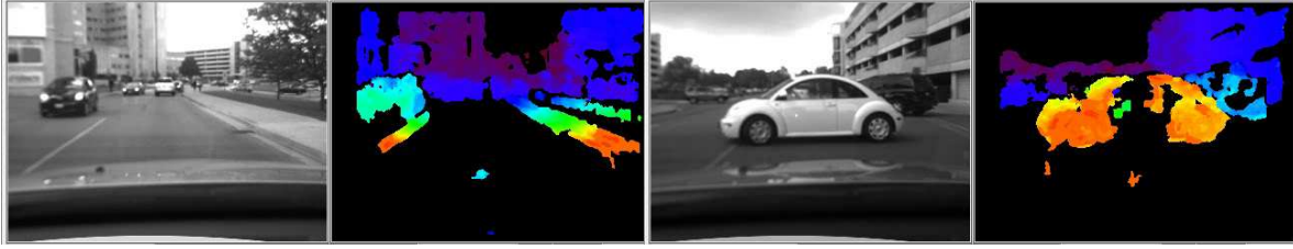
Fig. 3. Color-coded calibrated stereo depth maps are obtained at 30Hz. The distance between the instrumented vehicle and the roadside curbs, and other vehicles, is estimated in real-time.
