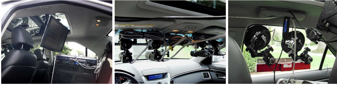
Fig. 5. The RoadLab in-vehicle laboratory: a) (left): on-board computer and LCD screen, b) (center): dual stereo front visual sensors, c) (right): side stereo visual sensors.
