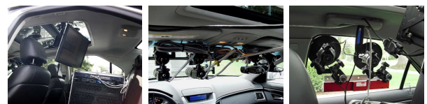
Fig. 1. The in-vehicle laboratory: a (left): on-board computer, b (center): front visual sensors, c (right): side visual sensors.
