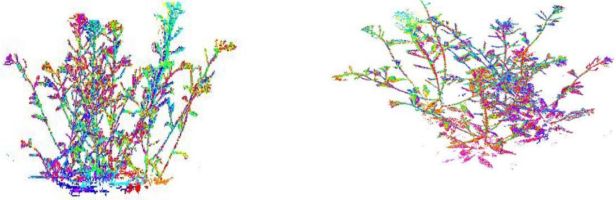
Figure 5. 12 scans captured in  $30^\circ$  increments about the plant and then merged into a single point cloud using MNN. Shown from two viewpoints, front facing on the left and from above on the right.
