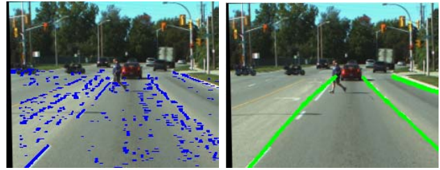
Fig. 2: a) (left): Lane features detected by Algorithm 1 b) (right): Projected lane splines on the image
