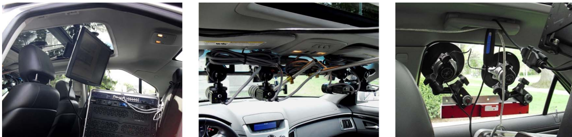
Fig. 4. RoadLAB in-vehicle laboratory. (a) (Left): on-board computer and LCD screen. (b) (Center): dual stereo front visual sensors. (c) (Right): side stereo visual sensors.
