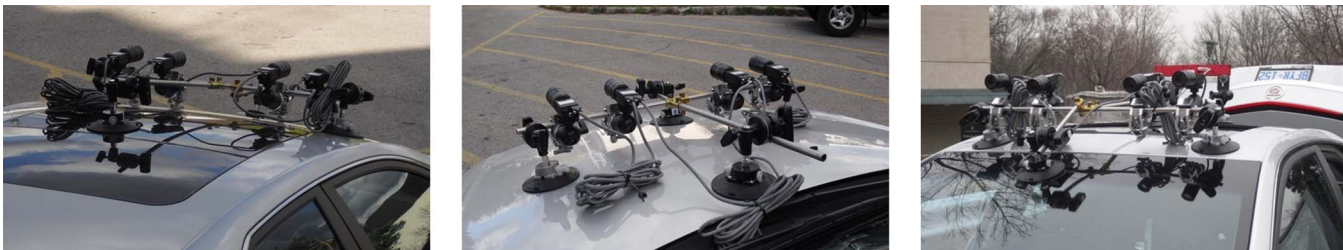
Fig. 5. Various mounting configurations. (a) (Left): dual stereo sensors mounted on top of vehicle. (b) (Center): dual stereo sensors mounted on hood of vehicle. (c) (Right): experiment with an external sensor configuration.
