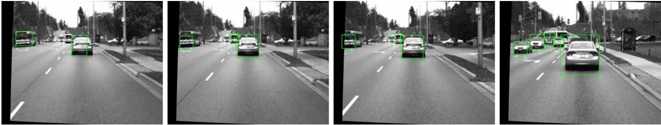
Fig. 10. Real-time vehicle tracking experiment using the RoadLAB instrumented vehicle in i-ADAS mode.
