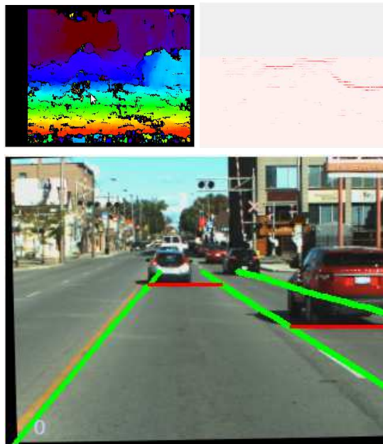
Figure 3: a)(top-left): Color-coded stereo depth map b) (top-right): Accumulated projected obstacle points c) (bottom): Obstacle-free area detection
