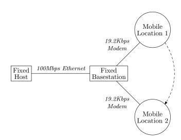
Figure 5: Network topology used for migration experiments
