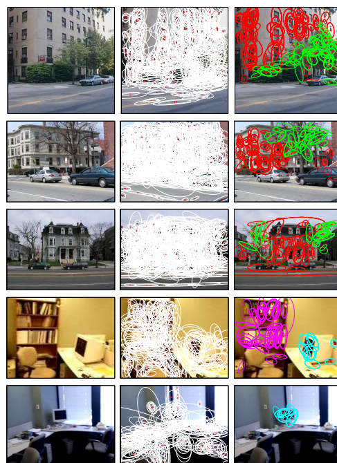
Figure 9: Example segmentations on the MIT dataset for the 10 topic decomposition. Left: the original image. Middle: all detected regions superimposed. Right: the topic induced segmentation. Only topics a, b, c and d from figure 8 are shown. The color key is: a-red, b-green, c-cyan, d-magenta. Note each image is segmented into several ‘topics’.
