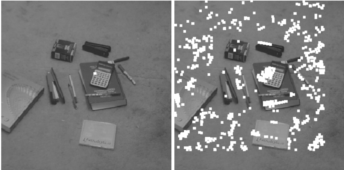
Figure 10: An example of detection of pocket calculator in real images. Eight anti-face detectors were sufficient to recover the calculator, without false alarms. A typical result is on the left. The eigenface method required a face space of dimension 30, to recover the calculator without false alarms. With a face space of dimension eight, there were many false alarms for the eigenface method (right).
