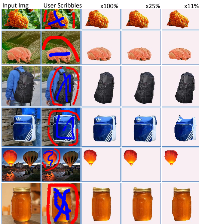
Fig. 9. Robustness to scale: segmentation results obtained for original images and their 25% and 11% scaled versions. We used \omega = 10 and 16 bins per color channel in all experiments. User scribbles were scaled accordingly for each experiment.
