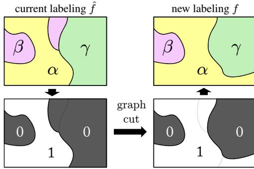
**Fig. 1** In an  $\alpha$ -expansion move, each location  $p$  is given a binary choice: keep its current label  $\hat{f}_p$  or switch to label  $\alpha$ . Here we use **1** to indicate a variable that decided to take label  $\alpha$ . Because variables interact through  $V$ , the binary decisions are inter-dependent and so the optimal move is calculated by a graph cut.
