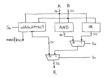
One possible ALU implementation. Do all of the operations, and control signal just controls a MUX to output.
