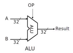
The control signal **OP** determines which arithmetic or logical operation is actually performed.
