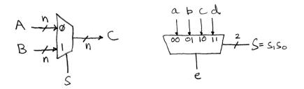
The control signal  $\mathbf{S}$  determines which input is used to set the output.
