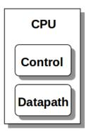
**CPU/Processor:** The encapsulation of the "working" part of the computer. Performs all the math, arithmetic, thinking, etc.
