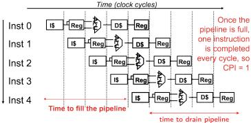
Potential speed-up via parallelism is equal to the number of stages.
