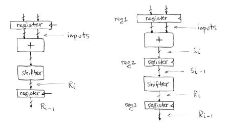
Break up a combinational circuit, reduce propagation delay, insert a register to store intermediate results, increase clock frequency.
