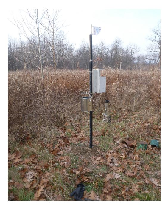
Weather station is now ready for winter data collection: addition of snow gauge (silver pail) completes instrumentation (such as it is): weather vane/velocimeter at top (bad design), hooded thermometer set (in white box), rain gauge in background. Barometric pressure and humidity are garnered from the Weather Network (Wardsville). We have accumulated over 800 sets of observations, from 2000 to 2012.
