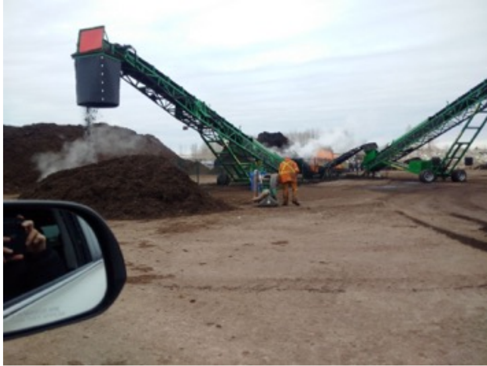
Completed compost is conveyed to a mound that awaits delivery to various end-users. Note steam caused by microbial heat generation.
