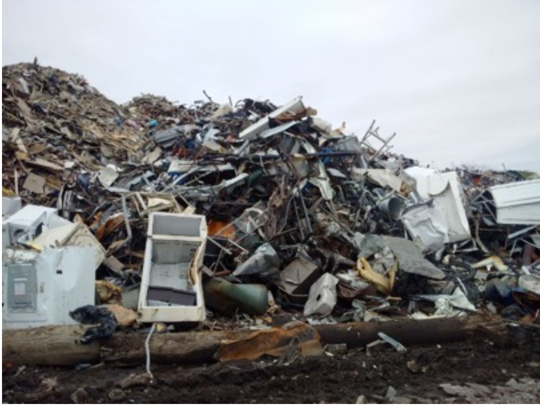
A small mountain of scrap wood and metal awaits processing at the beginning of the recycling process. Materials in this pile are hand-sorted, with the wood, for example, being directed to the pile shown below.
