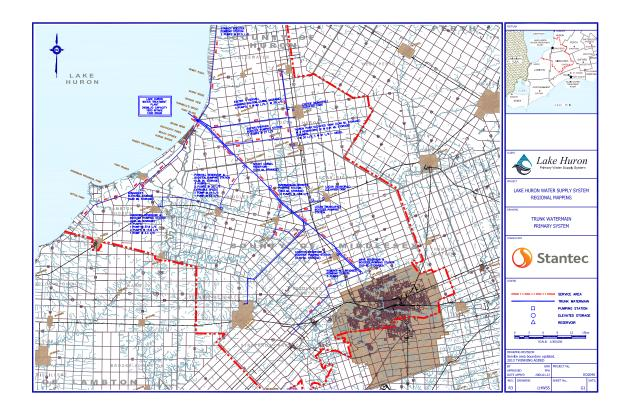
Distribution map for the Huron Water Supply operation shows the main 47 km pipeline (blue) that runs from Grand Bend to the Arva Reservoir and pumping station that serves the city. Boundaries of the supply system (red) are shared with adjacent water operations, including the Elgin system to the south that takes water from Lake Erie. (With apologies for the tiny print.)
