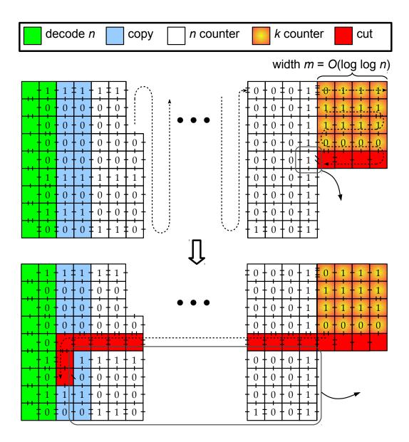
Figure 8: Tile system that produces a thin  $n \times k$  rectangle from the asymptotically optimal  $O(\sqrt{\log n})$  unique tile types. The different groups of tile types are listed left-to-right in the legend in the order they appear during assembly, and the arrows in the assembly help to illustrated when and where these tiles are placed.
