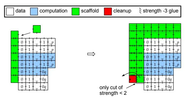
Figure 6: Tiles that position the cleanup tiles. Here the "copy" tiles from Figure 5 are depicted in the same shade as the computation tiles; now that f(x) has been computed our goal is to remove all of them from the subassembly representing f(x). The order of growth of the scaffold tiles ensures that cleanup does not begin until all of f(x) is present.
