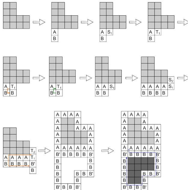
Figure 10. High-level design of another smart tile assembly system that replicates arbitrary shapes, and which uses a method similar to the smart sand robotic system replication of shapes (6).
