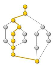
Assuming all strands run in unit time, the longest path in the DAG is equal to  $T_{\infty}$ . For this reason,  $T_{\infty}$  is also referred to as the **critical path length**.
