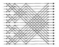
**Theorem.** Assume  $S \ge 3$ . For the n-point FFT graph we have  $Q \log(S) \in \Omega(n \log(n))$ . Moreover, there is a pebbling strategy for which  $Q \log(S) \in \Theta(n \log(n))$  holds.
