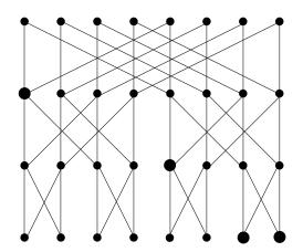
We have  $S_{\min}=4$ . More generally, for the FFT graph on  $n=2^k$  inputs we have  $S_{\min}=k+1$ .
