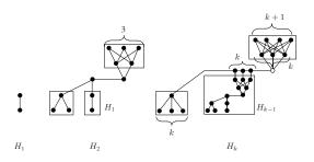
For  $k \ge 3$ , the grap  $H_k$  is of a k- input tree, T(k), a **spine**, S(k), of k vertices connected to the k outputs of  $H_{k-1}$ , an **open** vertex, and a complete bipartite graph BP(k), with k inputs and k+1 outputs.
