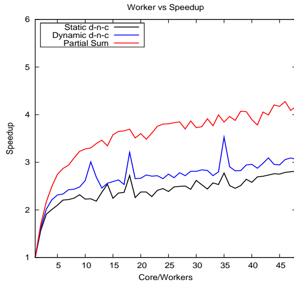
Figure 6.5: Speedup comparison between static divide and conquer, dynamic divide and conquer and Partial sum for degree 25000 PSnd polynomial.
