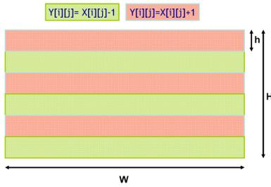
Figure 1: This figure shows a color-coding of the regions corresponding to increment and decrement operations in  $Y$  while executing the nested loops in routine 3.1. The orange colored regions indicate increment operations and green-colored regions represent decrement operations.
