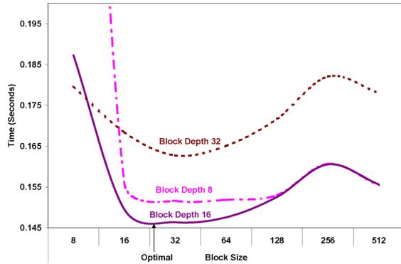
Figure 8: The performance of our cache-efficient matrix multiplication algorithm as a function of tile size for multiplying two  $2K \times 2K$  floating point matrices using a 7800 GTX GPU. We obtained the best performance using  $T \times T = 64 \times 64$  tiles and a depth of 16. As the block depth decreases, the vertex overhead dominates the memory bandwidth savings. The performance at  $T = D = 32$  degrades due to increase in time due to more fragment operations.
