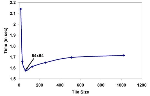
Figure 6: The performance of our cache-efficient sorting algorithm as a function of tile size sorting 8M floating point key-pointers using a 7800 GTX GPU.  $64 \times 64$  tiles had the best performance. As the tile size decreases, the vertex overhead dominates the memory bandwidth savings. As the tile size increases beyond  $64 \times 64$ , memory performance degrades due to cache misses.
