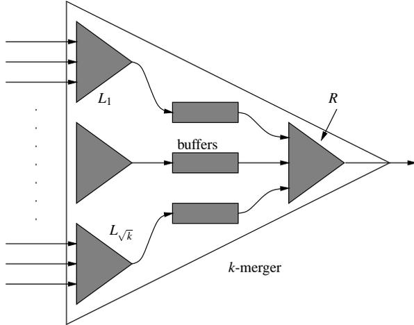
**Figure 3:** Illustration of a  $k$ -merger. A  $k$ -merger is built recursively out of  $\sqrt{k}$  “left”  $\sqrt{k}$ -mergers  $L_1, L_2, \dots, L_{\sqrt{k}}$ , a series of buffers, and one “right”  $\sqrt{k}$ -merger  $R$ .
