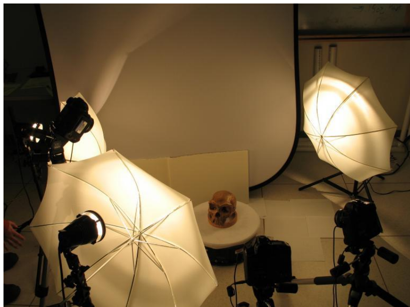
multi-view reconstruction set up
