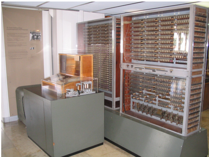
Konrad Zuse's Z3 electro-mechanical computer (1941, Germany). Turing complete, though conditional jumps were missing.
