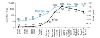
In complementary metal oxide semiconductor (CMOS) integrated circuit technology
