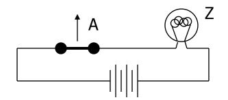
Open switch (if A is "0" or unasserted) and turn off light bulb (Z)
