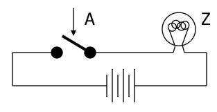
Close switch (if A is "1" or asserted) and turn on light bulb (Z)
