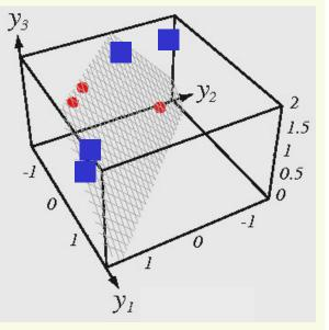
original feature space **x**; patterns are not linearly separable MNN finds nonlinear mapping  $\mathbf{y} = \boldsymbol{\varphi}(\mathbf{x})$  to 2 dimensions (2 hidden units); patterns are almost linearly separable
