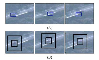
Figure 7: (A) The traditional mean-shift tracker is attracted to background pixels that have the same color as part of the tracked car, leading to tracking failure. (B) By modeling both object AND background color distributions, our tracking approach automatically down-weights shared colors, thus avoiding temptation.
