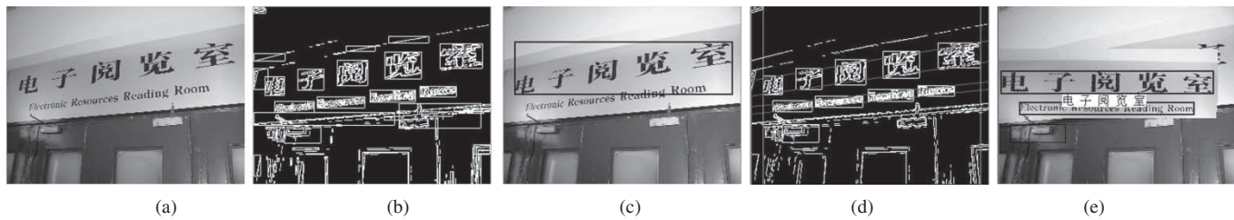
Fig. 19. Example of automatic sign detection and recognition.
