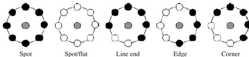
Fig. 4. Examples of texture primitives which can be detected by LBP (white circles represent ones and black circles zeros) [30].
