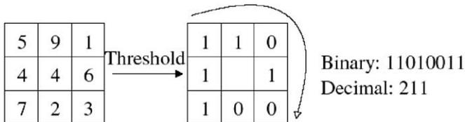
Fig. 3. The basic LBP operator [29].
