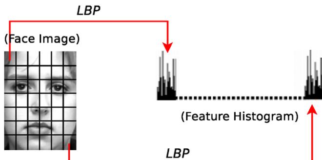
Fig. 6. A face image is divided into small regions from which LBP histograms are extracted and concatenated into a single, spatially enhanced feature histogram.
