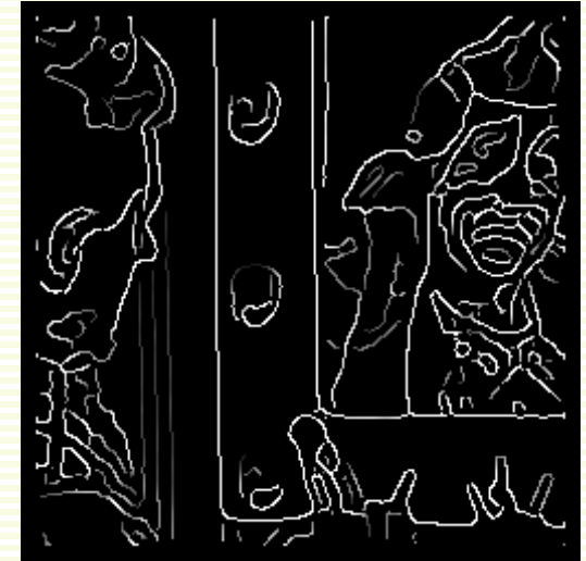
Canny with \sigma = 2
