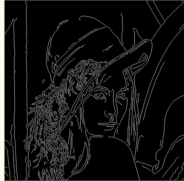
hysteresis with low and high thresholds
