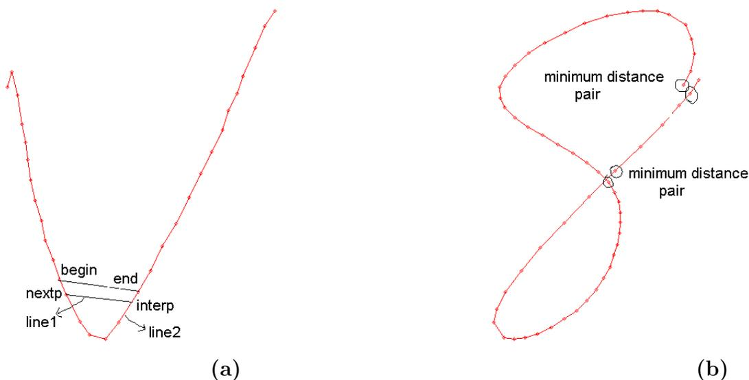
Figure 7: (a) Example 1 for Loop Detection (b) Example 2 for Loop Detection
