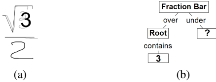
Figure 7. Partially recognized expression \sqrt{3} (a) and a corresponding layout tree (b)
