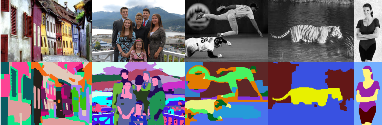
Figure 13. Unsupervised segmentation by clustering simultaneously over pixels and colour space using Gaussian Mixtures (colour images) and non-parametric histograms (greyscale images). Notice we find coarser clustering on baseball than Zabih & Kolmogorov [41] without over-smoothing. For segmentation, our energy is closer to Zhu & Yuille [42] but our algorithm is more powerful than region-competition.
