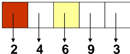
Interchange the smallest element with the one at the first position of the array
