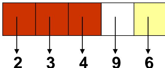
**Interchange the smallest element with the one at the third position**
