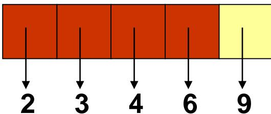
**Interchange the smallest element with the one at the fourth position**
