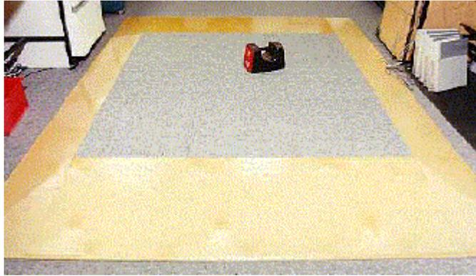
*Figure 5 Prototype Active Floor with test weight.*
