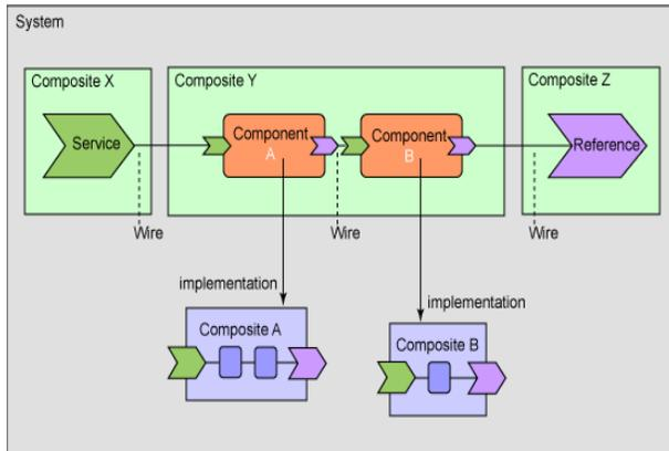
**Figure 4. Service Component Architecture [12]**
