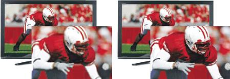
The image on the left simulates the picture resolution of an old-fashioned TV, while the image on the right simulates high-definition TV. Notice the soft edges and jagged lines in the non-HD image.
