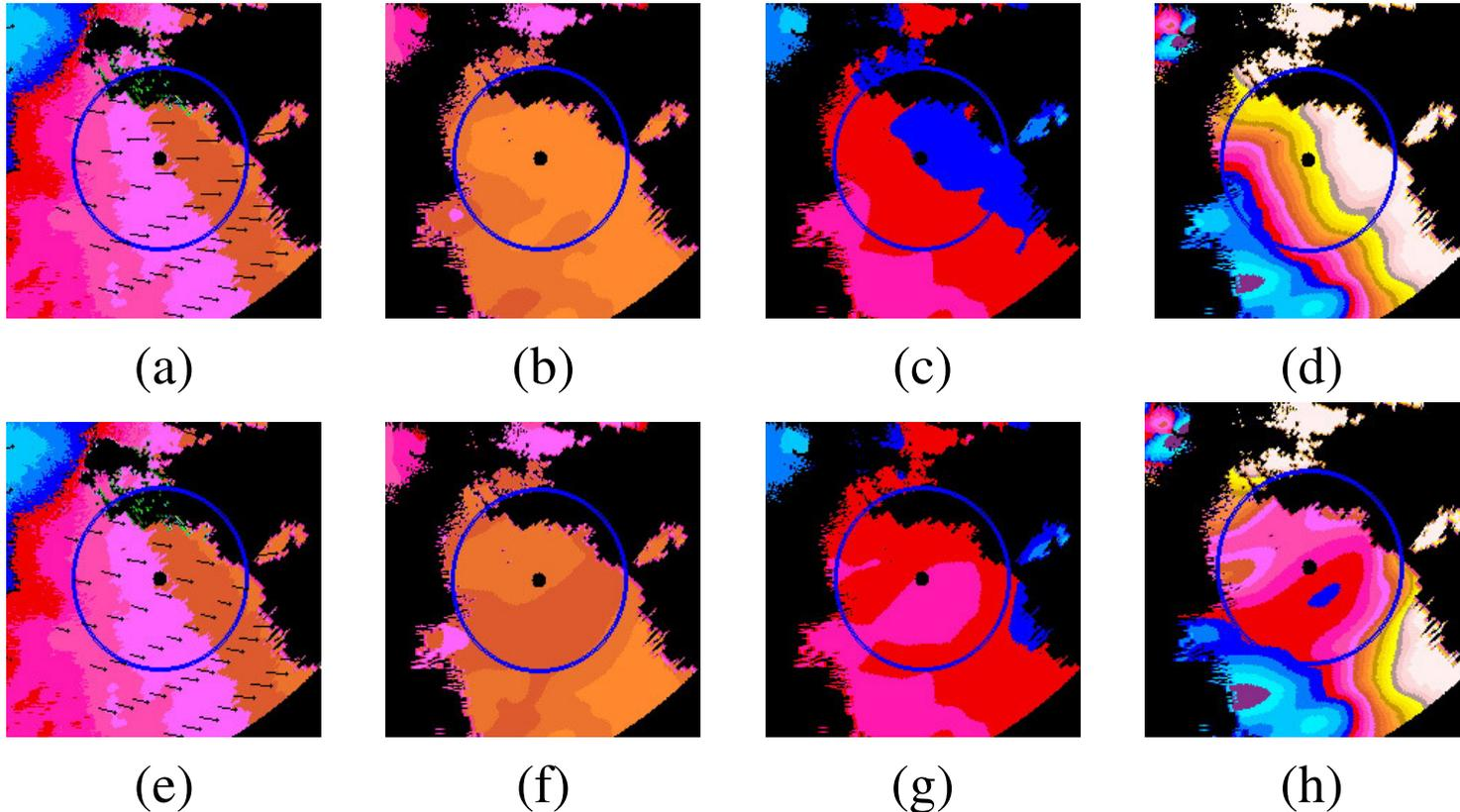
Full velocity retrieved from the Detroit Doppler (and the Harrow Windprofiler) data on August 19<sup>th</sup>, 2007 at 12:35:10: (a) the unrefined  $UV$  optical flow, (b) the  $U$ , (c)  $V$  and (d)  $W$  components of the unrefined optical flow, (e) the refined  $UV$  optical flow and (f) the  $U$ , (g)  $V$  and (h)  $W$  component of the refined optical flow.
