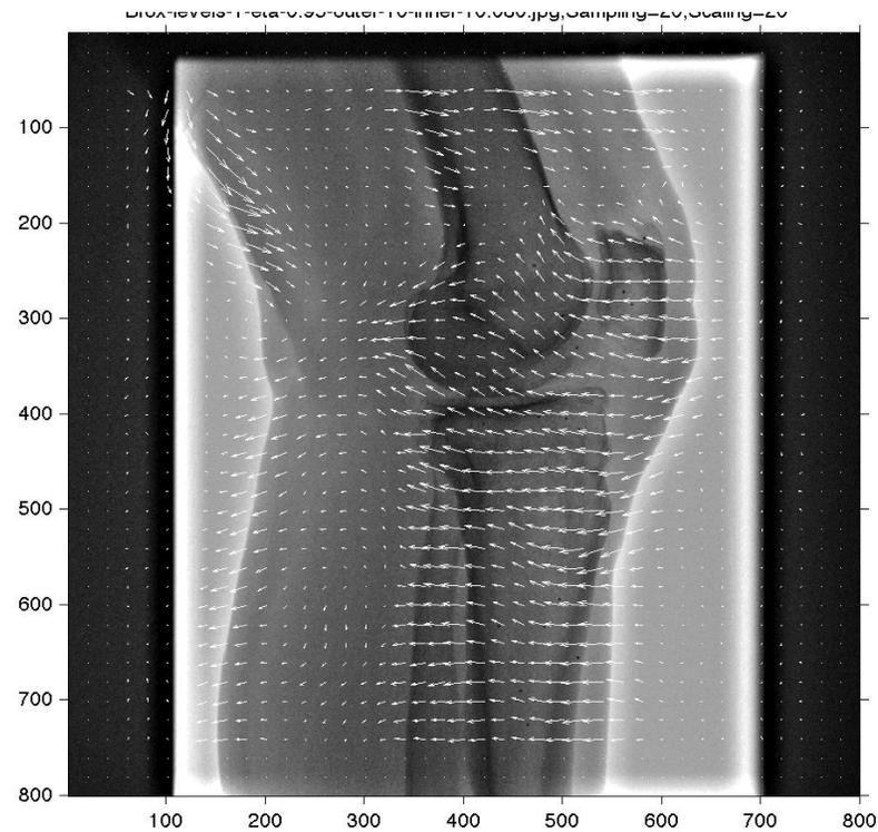
2D Optical Flow on image 80 in a fluoroscopic image video of a bending knee.
