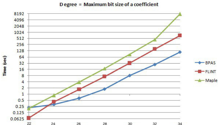
Figure: BPAS (parallel) vs FLINT (serial) vs Maple 18 (serial) with the logarithmic scale in radix 2 of the maximum bit-size of an input polynomial as the horizontal axis.
