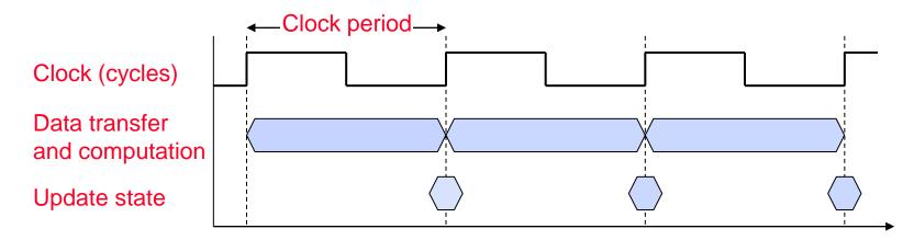
Clock period (cycle): duration of a clock cycle
