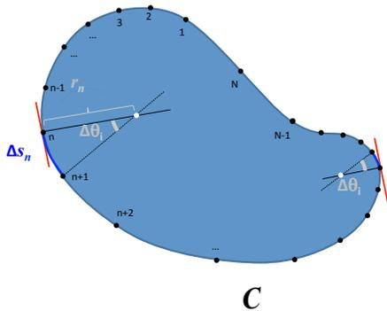
Figure 2. The partial sum approximation (3) of the integral  $\int_C \kappa^2 ds$  uses a sequence of points on the contour  $C$ . Our approach is to select all contour points  $\{n\}_1^N$  where the tangent is consistent with the orientation of some triple clique in a given neighborhood in Figure 3(a). For example, two points in this Figure are marked with a tangent of the same orientation as clique  $c_i$  in Figure 3(a). Each point  $n$  corresponds to a particular clique index  $i(n)$ .
