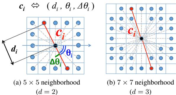
Figure 3. Neighborhood systems of size  $(2d+1) \times (2d+1)$  for (a)  $d = 2$  and (b)  $d = 3$ . To make all triple cliques approximately the same length, for each orientation  $\theta_i \in \Theta$  we select the centered triple clique  $c_i$  whose length  $d_i$  is as close to  $d$  as possible.  $\theta_i$  indicates the orientation of  $c_i$  with respect to the horizontal axis.  $\Delta\theta_i$  denotes the angular rotation to the next clique.
